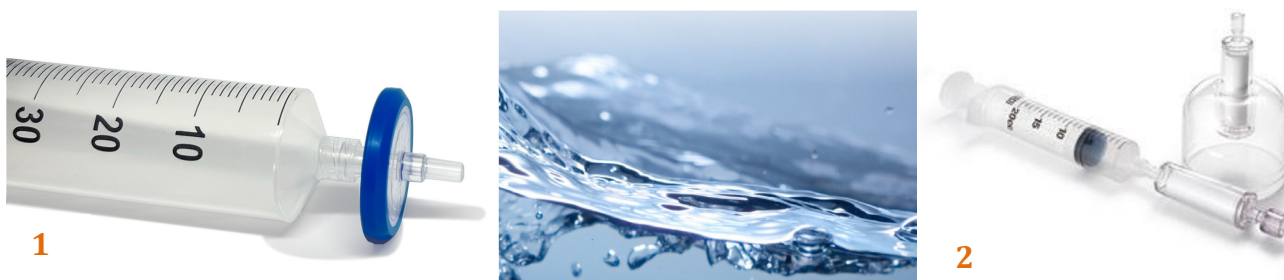
1: MCE-filter for virus. 2: Sterivex-filter for bakterier.
